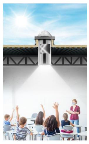
sunlight from various angles. These domes serve as a gateway for harnessing natural daylight. The captured sunlight is then channeled into the building through highly reflective tubes, ensuring maximum efficiency. Within the building space, the light is diffused by fixtures, resulting in a beautiful and evenly spread illumination of natural daylight.
