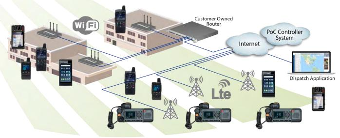
The PoC devices on the nationwide 4G/LTE network (lower right of the diagram) use SIM cards to access the mobile operator's cellular network with an Access Point Name (APN) that routes the data traffic to the mobile operator's internet gateway. The PoC devices on the 4G/LTE network include mobile PoC radios installed in vehicles, in addition to the same devices as on the Wi-Fi network. The PoC controller accesses the internet through the customer's network router.
